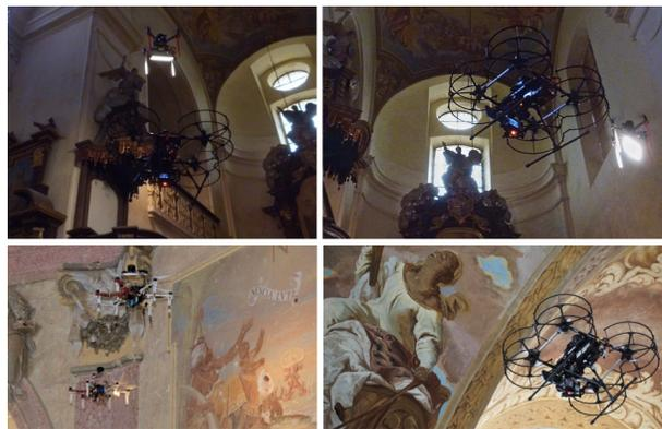
Fig. 1: An example of formations used in the task of cooperating smart lighting in the restricted environment of the interiors of historical buildings.
