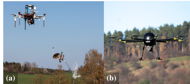
Fig. 15: Development of the Eagle.One autonomous aerial interception system based on the MRS hardware platform: (a) First prototype using the MRS UAV platform during a successful interception. (b) Second prototype designed by the MRS team specifically for Eagle.One project. Video: https://youtu.be/hEDGE7oFX1c .
