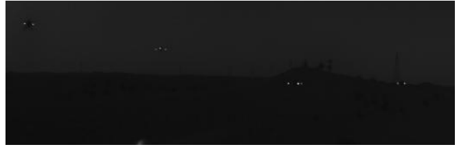
Fig. 3: View from onboard ultraviolet-sensitive cameras used in the UVDAR system. Note the clarity of the onboard LED markers of neighboring UAVs, despite this image being captured at midday in a desert setting.
