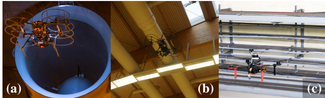
Fig. 10: Snapshots of deployment of industrial platforms (a, b) and a general research platform (c) for inspection of ventilation systems, structural degradation, and electrical infrastructures in tunnels, halls, and storage houses. Video: https://youtu.be/60nKXamV2ds .
