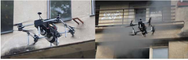
Fig. 16: Extinguishment of fires in above-ground floors by launching fire-extinguishing capsules into the thermal sources. Multimedia is available at https://youtu.be/QHpifXJzH5g .
