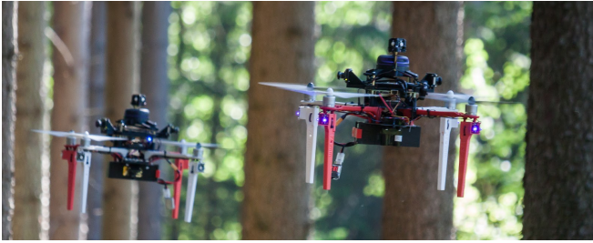
Fig. 2: A pair of DJI F450-based UAV platforms equipped with the UVDAR system. Note the ultraviolet LEDs and dual cameras on the sides of the UAV body.
