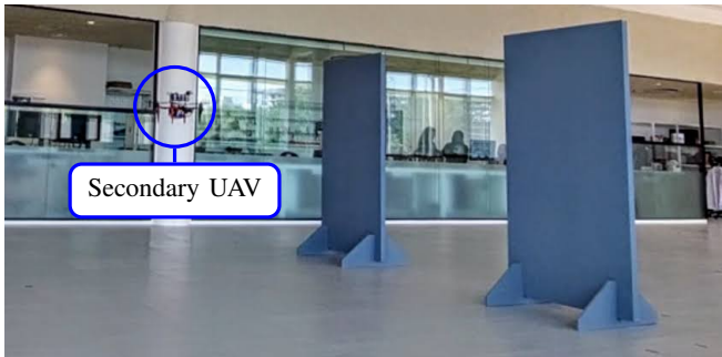
Fig. 8: Experimental evaluation of flight between obstacles. The primary UAV guided the secondary UAV to pass through a gap between two rectangular panels.
