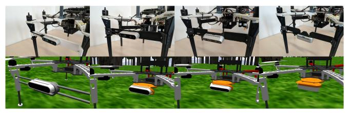
Fig. 2: Camera mounting position between the front legs of the real UAV (top row) and the simulated (bottom row) UAV model. The orientations of the camera considered in this paper are depicted from left to right in this order:  $0^{\circ}$ ,  $10^{\circ}$ ,  $30^{\circ}$  and  $90^{\circ}$ .
