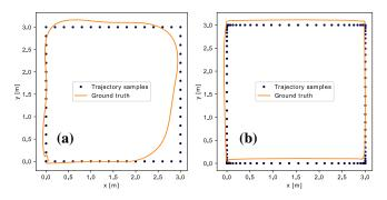
Fig. 4: Trajectory with constant velocity profile (a) violates acceleration constraints during the UAV flight. The UAV platform used in this flight is described in Sec. IV-C. The smoothed trajectory (b) is constrained to  $0.4 \text{ m s}^{-2}$ , which improves tracking precision, and prevents aggressive tilting that would result in losing image features.
