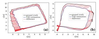
Fig. 7: Trajectories flown with SVO in the feedback of the control system with  $0^{\circ}$  camera orientation. ATE of 1.3395 m was achieved on trajectory (a) with  $0.5 \text{ m s}^{-1}$  desired velocity. Faster trajectory (b) with  $1 \text{ m s}^{-1}$  desired velocity reached 1.3038 m ATE.
