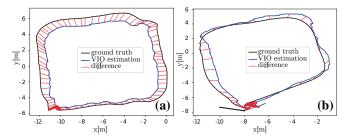
Fig. 9: Trajectories flown with S-MSCKF in the feedback of the control system. Figure (a) shows trajectory for  $0^{\circ}$  camera orientation,  $1 \text{ m s}^{-1}$  desired velocity with 0.7574 m ATE. Figure (b) shows trajectory for  $90^{\circ}$  camera orientation,  $3 \text{ m s}^{-1}$  desired velocity with 0.4617 m ATE.
