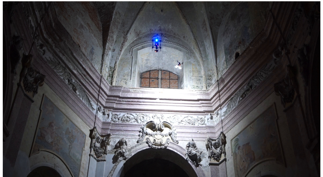
Figure 7. Applying Reflectance Transformation Imaging documentation technique in the Church in Stará Voda. The unmanned aerial vehicle carrying the camera (equipped with a blue indication diode) is hovering in front of the vault located approximately 12 m above the ground while the unmanned aerial vehicle equipped with light is flying through predefined positions to provide lighting from all-around directions.
