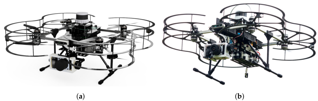
Figure 1. The hardware platform application-tailored for deployment in interiors of historical structures. The platform is designed with a high emphasis on motor and sensory redundancy, robust and stable flight, and minimal dimensions with maximal payload weight. (a) CAD model. (b) Real-world platform.
