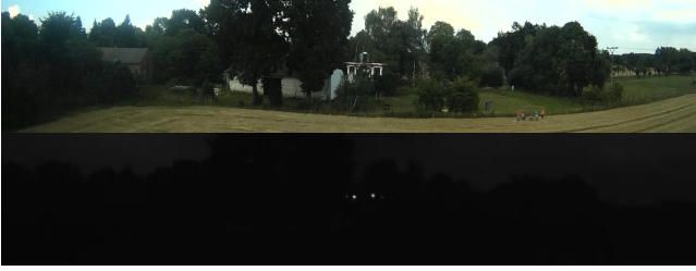
Fig. 2: Comparison between visible and UV camera footage from UVDAR, collected during the experiment. The UV image is significantly easier to process to retrieve UAV information.
